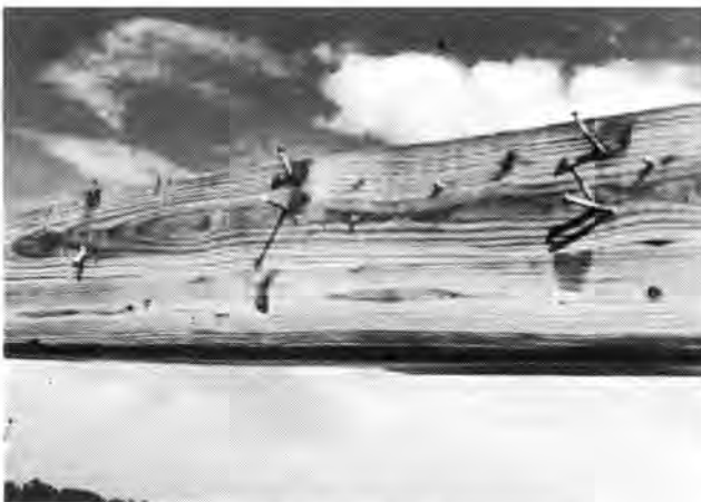
Figure 4.26. Toe Nailing Provides Limited Pull-Out Resistance
